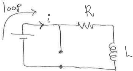
Outer Loop Clockwise:  $V - iR - L \frac{di}{dt} = 0$
