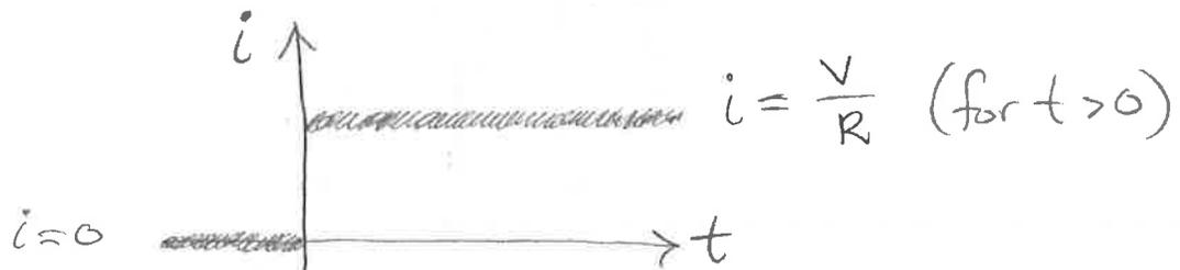
⊗ This would produce an infinite value of  $\frac{di}{dt}$  and therefore an infinite induced opposing electromotive force in the inductor:  $\mathcal{E}_{\text{ind}} = -L \frac{di}{dt} = -\infty$ .
