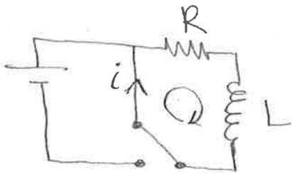
Current continues flowing clockwise immediately after switch is flipped.
