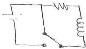
Key Point: Inductors prevent discontinuous changes in current since then  $\mathcal{E}_{\text{ind}} = -L \frac{di}{dt} \rightarrow \infty$ .
