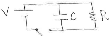
Capacitor will discharge through resistor R.
