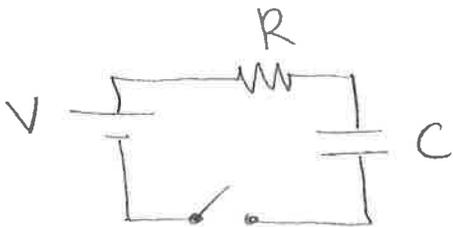
Suppose at  $t=0$  switch is closed.
