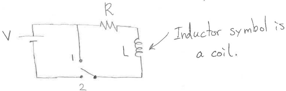
At time  $t=0$  we flip the open switch to position 2.
