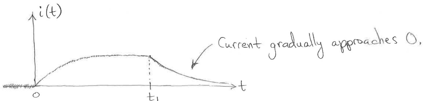
⊛ The battery is disconnected, so where does the energy come from to sustain current after switch is flipped?
