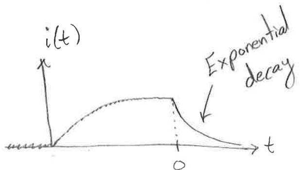
⊗ Note that for both differential equations, we needed an "initial condition" (that is, the value of the current before the switch was flipped)
