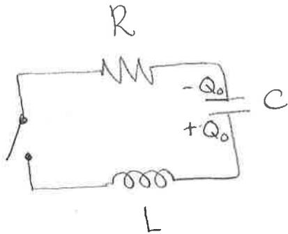
The capacitor starts out charged ( $+Q_0$ ) and at time  $t=0$  the switch is closed
